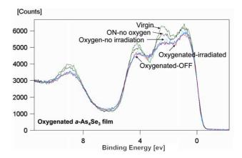
Fig. 6. XPS data of the valence band of the virgin, oxygenated a- $As_4Se_3$  film for the ON–no oxygen, oxygenated–unirradiated, oxygenated–ON(1) and oxygenated–OFF irradiation states.
