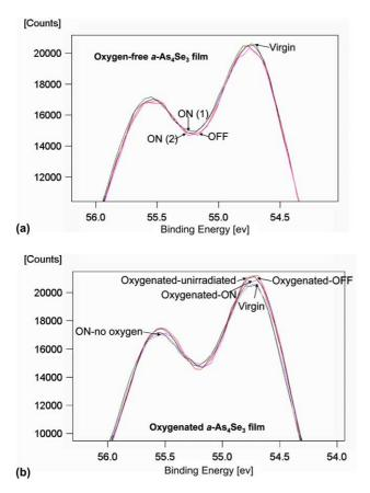
Fig. 3. (a) Details of Se 3d core levels in the oxygen-free a-As<sub>4</sub>Se<sub>3</sub> film for the Virgin, ON(1), OFF and ON(2) irradiation states. (b) Details of the Se 3d core levels in the oxygenated a-As<sub>4</sub>Se<sub>3</sub> film for the Virgin, ON–no oxygen, oxygenated–unirradiated, oxygenated–ON(1) and oxygenated–OFF irradiation states.
