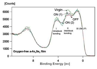
Fig. 5. XPS data of the valence band spectra of the virgin, oxygen-free  $a-As_4Se_3$  film for the ON(1), OFF and ON(2) irradiation states.
