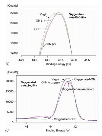
Fig. 4. (a) Details of the As 3d core levels in the oxygen-free  $a-As_4Se_3$  film for the Virgin, ON(1), OFF and ON(2) irradiation states. (b) Details of the As 3d core levels in the oxygenated  $a-As_4Se_3$  film for the Virgin, ON–no oxygen, oxygenated–unirradiated, oxygenated–ON(1) and oxygenated–OFF irradiation states.
