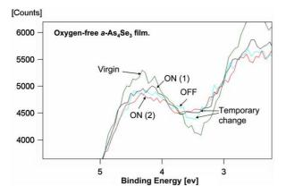
Fig. 7. XPS data of the valence band of the oxygen-free a-As<sub>4</sub>Se<sub>3</sub> film showing reversible change after turning the light OFF.
