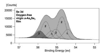
Fig. 1. XPS spectrum showing Se3d core level for oxygen-free  $a-As_4Se_3$  virgin film. 1, 2 and 3 represent the components of the spectrum for Se atoms with corresponding coordination number.
