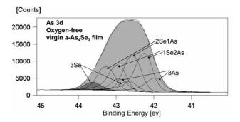
Fig. 2. XPS spectrum showing As 3d core level for oxygen-free  $a-As_4Se_3$  virgin film. The deconvoluted peaks are labeled showing the nearest neighbor atoms.
