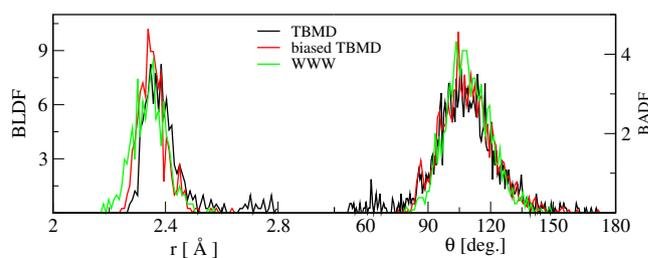
**Figure 2.** Bond-length (left) and bond-angle (right) distributions of *a*-Si from three models: biased TBMD, TBMD, and WWW<sup>7</sup>.
