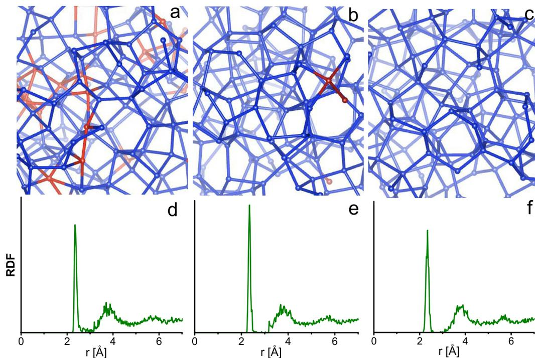
**Figure 1.** (a–c) The structural features of the TBMD, biased TBMD and WWW models of *a*-Si respectively. Mis-coordinated atoms and their bonds are visualized in red and normally coordinated atoms are in blue. Cutoff radius of 2.8 Å was used to define a bond for all three models. (d–f) Radial distribution function (RDF) of these models are plotted in the same order.
