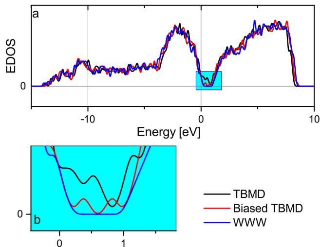
**Figure 3.** (a) Electronic Density of states (EDOS) for three models of *a*-Si: TBMD, biased TBMD and WWW<sup>7</sup>. (b) The density of states in the gap region is highlighted.
