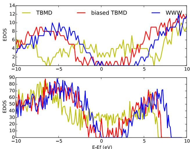
**Figure 5.** Density of electronic states (EDOS) for three models of *ta*-C: TBMD, biased TBMD and WWW<sup>7</sup>. The upper plot is obtained using the tight-binding model of ref. 22 and the lower one is obtained from density functional theory (DFT) calculations<sup>11,12</sup>.
