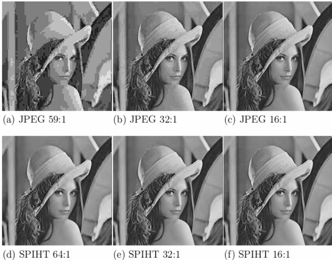
Figure 2-6: An image is compressed using a Fourier-based JPEG scheme (not to be confused with the wavelet-based JPEG2000) at different compression ratios in (a)-(c). The same image is compressed using the wavelet-based SPIHT scheme in (d)-(e). Note that there is almost no apparent loss in the wavelet compression even at a 64 times reduction in file size. (Source: [17].)
