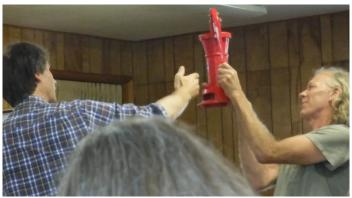
Notice that when you push down on the handle, a plunger inside lifts a column of water which then pours out the spout, and also draws more water up from the reservoir below via suction. When you push the handle up, a check valve opens and the plunger goes down into the column of water. As you move the handle up and down, spurts of water come out the spout.
