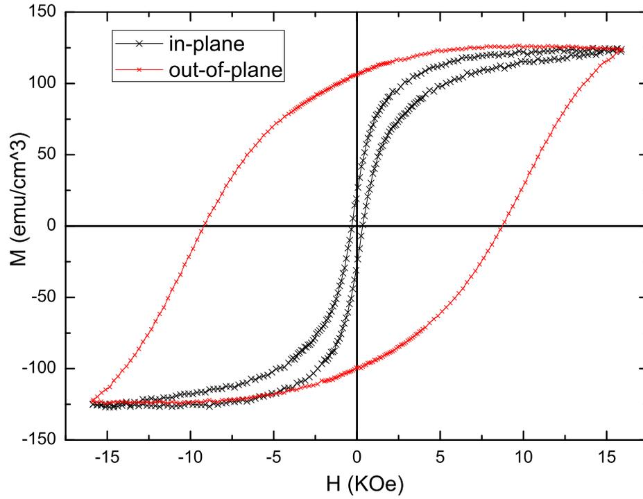
FIG. 4: Magnetization as a function of applied magnetic field with the field applied parallel and perpendicular to the  $\delta\text{-Mn}_3\text{Ga}_2(001)$  film surface. Measurements were made with vibrational sample magnetometry at room temperature ( $27^\circ\text{C}$ ).
