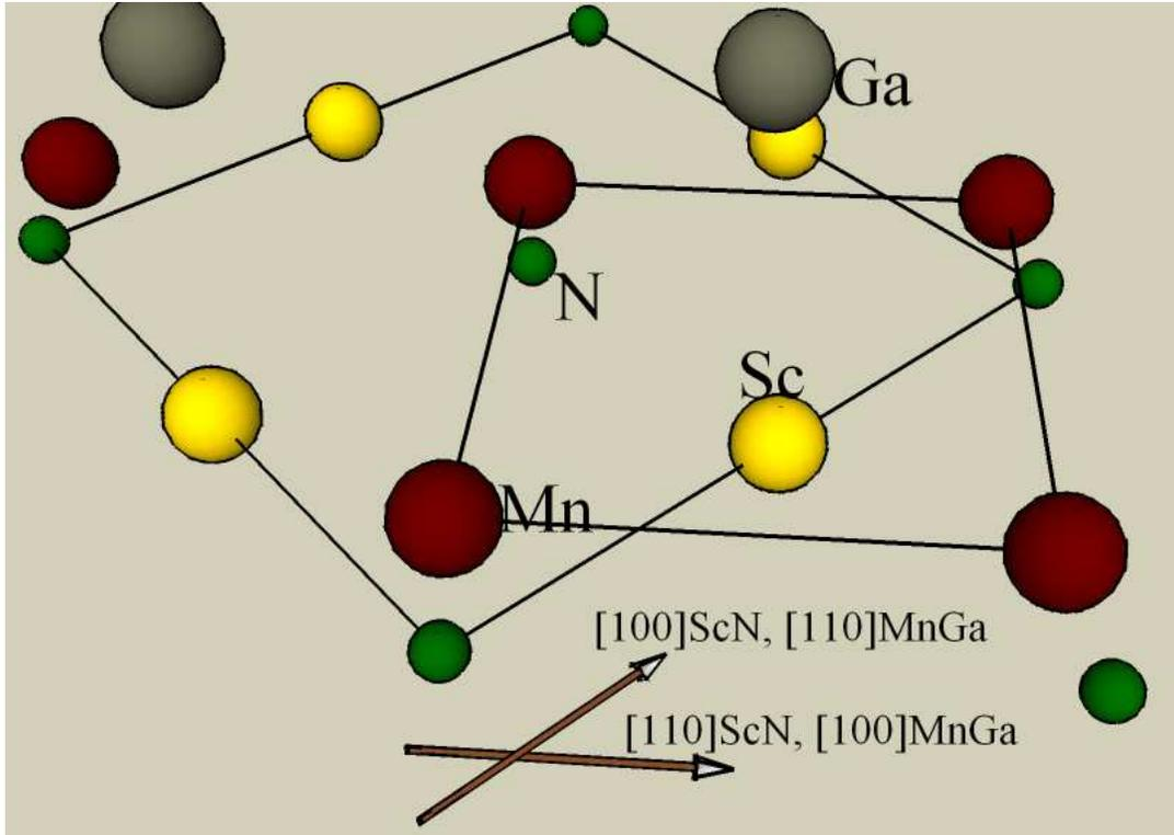
FIG. 2: 3D schematic showing derived epitaxial relationship of  $\delta$ -MnGa(001) to ScN(001). Squares indicate the conventional unit cells of the two lattices.
