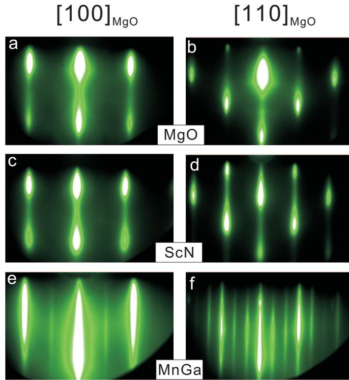
FIG. 1: RHEED patterns: left column along  $[100]$  of  $\text{MgO}(001)$ ; right column along  $[110]$  of  $\text{MgO}(001)$ . (a),(b)  $\text{MgO}(001)$  after annealing, taken at  $750^\circ\text{C}$ . (c),(d) 10 nm  $\text{ScN}(001)$  grown at  $750^\circ\text{C}$ . (e),(f) 130 nm  $\delta\text{-Mn}_3\text{Ga}_2$  grown at  $T_S = 250^\circ\text{C}$ . Note that the direction has now changed to  $[110]_{\text{MnGa}}$  and  $[100]_{\text{MnGa}}$  for (e) and (f), respectively.
