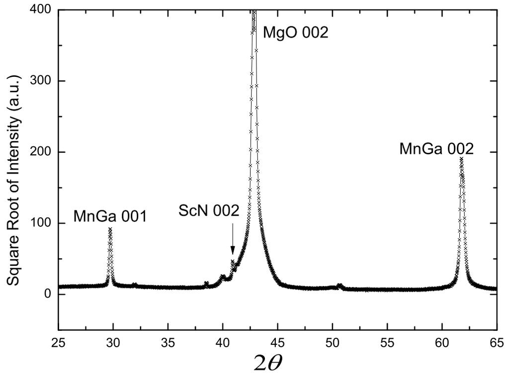
FIG. 3:  $\theta$  to  $2\theta$  X-ray diffraction spectrum acquired on  $\delta$ -MnGa film grown on ScN/MgO(001).
