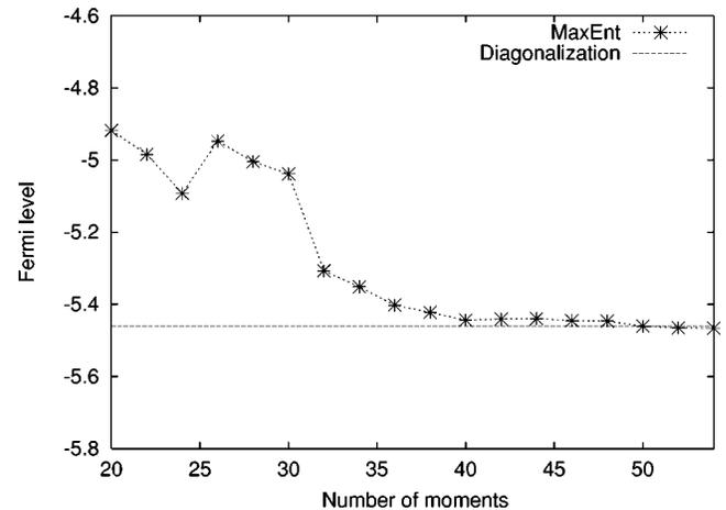
FIG. 3. Fermi level of amorphous silica as a function of number of the shifted Chebyshev moments. The value obtained from direct diagonalization of the Hamiltonian matrix is  $-5.465$  eV and is plotted as a horizontal line in the figure.
