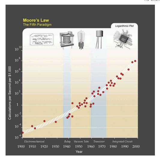
Kurzweil expanded Moore's law from integrated circuits to earlier transistors, vacuum tubes, relays, and electromechanical computers to show that his trend holds there as well.
