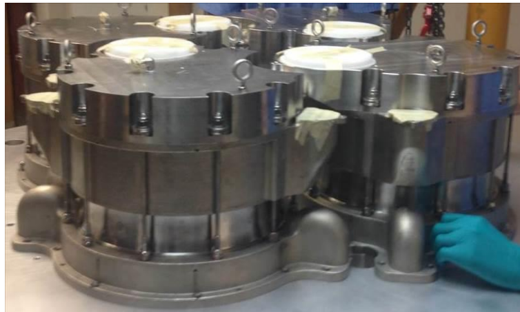
Figure 5. Four thermodynamic circuits fully assembled onto the cold plate.
