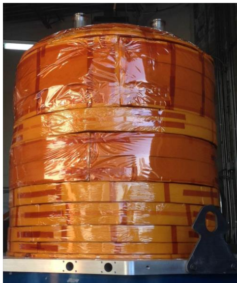
Figure 13. Insulated hot side of the 25 kW ThermoHeart Engine
