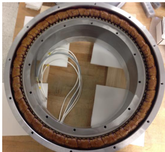
Figure 11. Permanent magnet alternator prior to installation.
