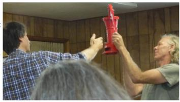
Notice that when you push down on the handle, a plunger inside lifts a column of water which then pours out the spout, and also draws more water up from the reservoir below via suction. When you push the handle up, a check valve opens and the plunger goes down into the column of water. As you move the handle up and down, spurts of water come out the spout.
