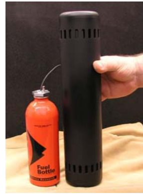
Figure 8 Mass-optimized Palm Power system
