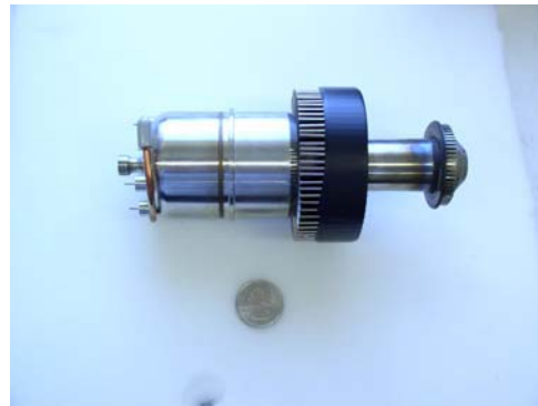
Figure 4 Hermetically-sealed 35 W_e engine, showing external acceptor and air-cooled rejector
