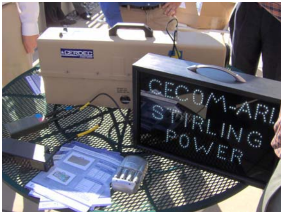
Figure 3 Battery Charger system demonstration
