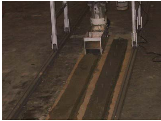
Figure 3. NIST Concrete Deposition Experiment
