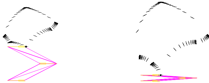
Figure 11. BAT Workspace 0.45L_0 \leq L_i \leq L_0 (left) and 0.415L_0 \leq L_i \leq L_0 (right)
