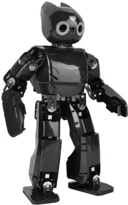
Figure 2: The DARwIn-OP 20-DOF humanoid robot. The shoulder has two rotational joints and the arm terminates with an elbow flexion joint. This model does not contain a robotic gripper.
