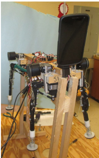
Figure 1b. RoboCat with Improved Legs
