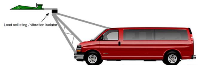
Figure 2. Windmobile Conceptual Design
