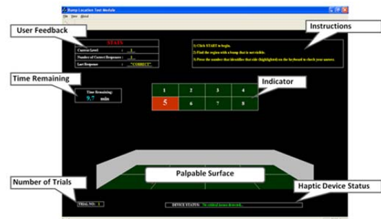
Figure 2. Sample screen layout for the haptic modules
