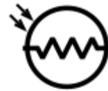
Photoresistor Schematic Symbol
