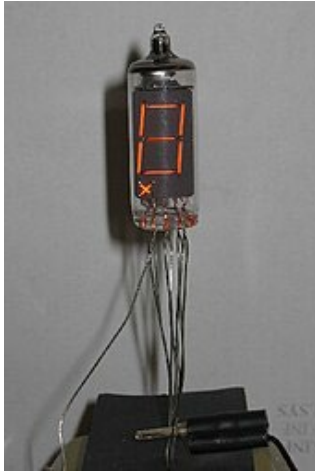
Seven-Segment Display showing 8
