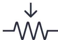
Potentiometer Schematic Symbol
