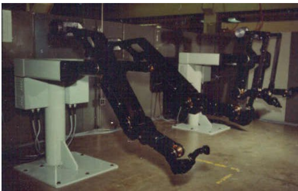
Laboratory Telerobotic Manipulator (LTM) SRMS with Flight Telerobotic Servicer (FTS)
