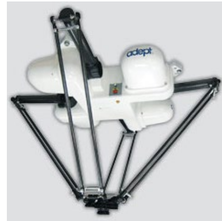
Adept Quattro Parallel Robot (Delta parallel robot) 4-RUU
