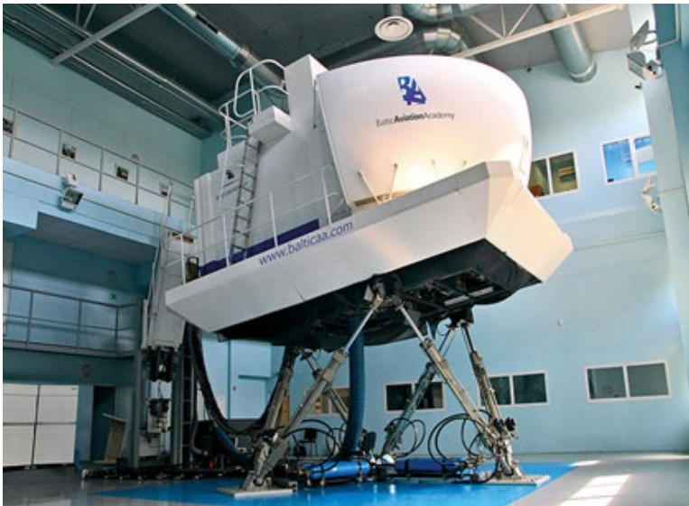
Airbus 320 Full Flight Simulator (Stewart Platform parallel robot) 6-UPS
