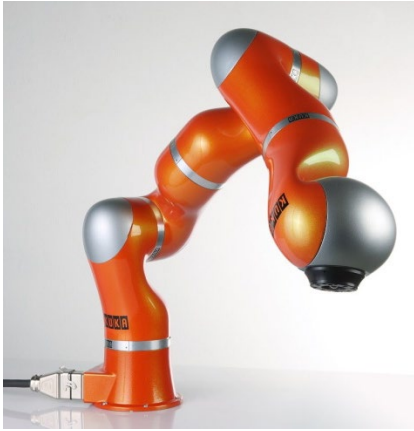
KUKA LWR 7R 7-dof serial robot
