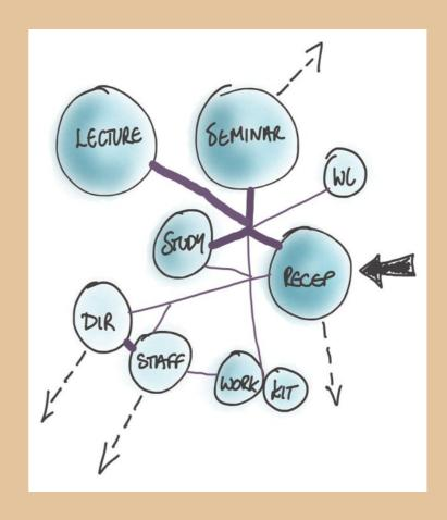
The bubble diagram helps make the connection between basic spatial requirements and a fully drawn out floor plan. It is a trial and error method of exploring configuration and relationship options.
